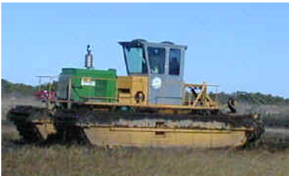
Figure 7 – Photo of specialized tracked vehicle clearing blocked mosquito ditches. These machines are capable of traveling over the marsh surface without damaging the fragile wetland vegetation.
